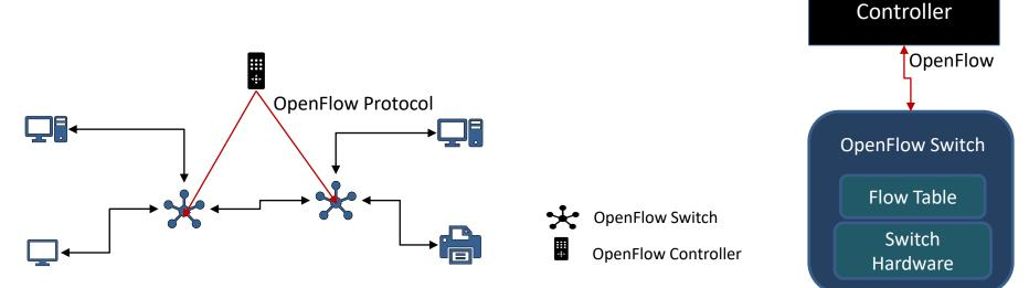
Courtesy: Nick McKeown et al. "OpenFlow: Enabling Innovation in Campus Networks", Open Networking Foundation "OpenFlow Switch Specification"
