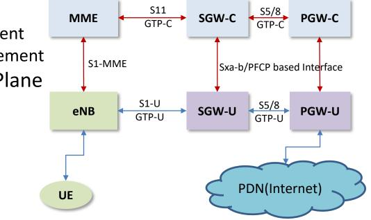
*Courtesy: 3GPP TS 23.214, "*Architecture enhancements for control and user plane separation of EPC nodes" *3GPP TS 29.244, "*Interface between the Control Plane and the User Plane Nodes"
