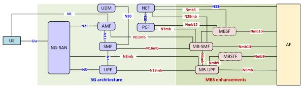
Fig. 1. 5G architecture with MBS enhancements [4]. AMF: Access and Mobility Management Function, AF: Application Function, MB-SMF: Multicast/Broadcast Session Management Function, MBSF: Multicast/Broadcast Service Function, MBSTF: Multicast/Broadcast Session Transport Function, MB-UPF: Multicast/Broadcast User Plane Function., NEF: Network Exposure Function, NG-RAN: Next generation Radio Access Network, PCF: Policy Control Function, UDM: User Data Management, and UE: User Equipment.
