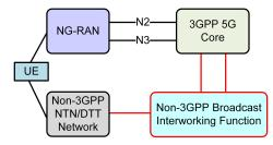
Fig. 7. Integration of non-3GPP broadcast network using a new interworking function. UE: User Equipment, NTN: Non-Terrestrial Network, DTT: Digital Terrestrial Technologies, and NG-RAN: Next Generation Radio Access Network.
