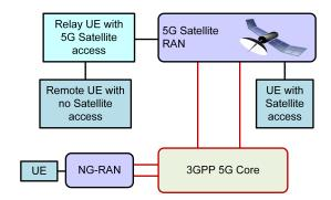
Fig. 5. Integration of satellite access based 5G-NR. NG-RAN: Next Generation Radio Access Network, RAN: Radio Access Network, and UE: User Equipment
