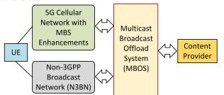
Fig. 8. MBOS for load sharing between 5G and non-3GPP broadcast networks. UE: User Equipment.
