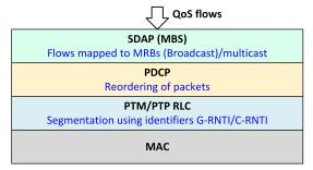
Fig. 4. Sublayers for 5G MBS NR [7]. MBS: Multicast/Broadcast Services, SDAP: Service Data Adaptation Protocol, MRB: MBS Radio Bearers, PDCP: Protocol Data Convergence Protocol, RLC: Radio Link Layer, G-RNTI: Group Radio Network Temporary Identifier, C-RNTI: Cell Radio Network Temporary Identifier, QoS: Quality of Service, PTM: Point-to-multipoint and PTP: Pointto-point.
