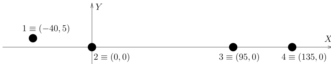
Figure 4.1: An STDMA wireless network with four nodes.
