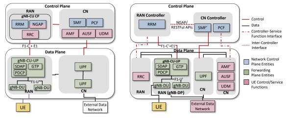
(a) Existing 3GPP 5G Network Architecture (b) Proposed 5G-Serv Architecture Fig. 1: Proposed 5G-Serv Architecture
