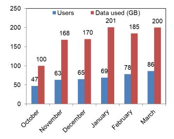
Fig. 4: Average number of active users and data usage pattern as observed in the Unlicensed band testbed from October 2017 - March 2018.
