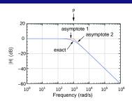
$$\text{Consider } H(s) = \frac{1}{1+s/p} \to H(j\omega) = \frac{1}{1+j\left(\omega/p\right)} \,, |H(j\omega)| = \frac{1}{\sqrt{1+(\omega/p)^2}} \,.$$
