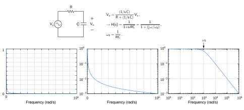
Since  $\omega$  and  $|H(j\omega)|$  vary by several orders of magnitude, a linear  $\omega$ - or |H|-axis is not appropriate  $\to \log |H|$  is plotted against  $\log \omega$ .
