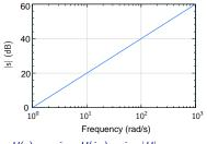
For H(s) = s, i.e.,  $H(j\omega) = j\omega$ ,  $|H| = \omega$ .  $\rightarrow 20 \log |H| = 20 \log \omega$ ,
