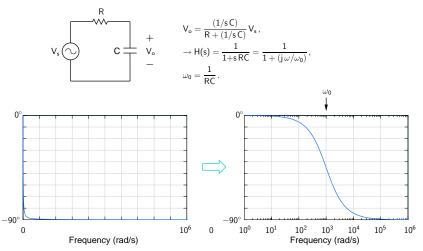
\* Since  $\angle H = -\tan^{-1}(\omega/\omega_0)$  varies in a limited range (0° to  $-90^\circ$  in this example), a linear axis is appropriate for  $\angle H$ .
