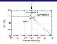
$$\text{Consider } \textit{H(s)} = \frac{1}{1 + s/p} \rightarrow \textit{H(j}\omega) = \frac{1}{1 + j\left(\omega/p\right)} \,, \left|\textit{H(j}\omega\right)\right| = \frac{1}{\sqrt{1 + (\omega/p)^2}} \,.$$
