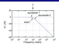
$$\text{Consider } \textit{H(s)} = \frac{1}{1 + s/p} \rightarrow \textit{H(j}\omega) = \frac{1}{1 + j\left(\omega/p\right)} \,, |\textit{H(j}\omega)| = \frac{1}{\sqrt{1 + (\omega/p)^2}} \,.$$
