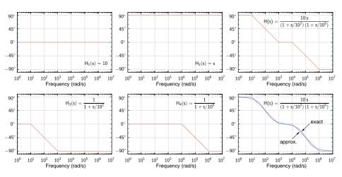
\* As we have seen, the contribution of a pole to the magnitude and phase plots is well represented by the asymptotes when  $\omega \ll p$  or  $\omega \gg p$  (similarly for a zero).
