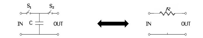
Two-phase non-overlapping clocks are used to control switches S1 & S2.
