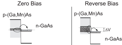
Figure 6.17: Scheme of the (abrupt) (Ga,Mn)As/GaAs p - n -diode structure used in the simplified tight-binding calculations at zero and reverse bias.
