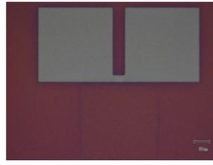
(e): After removal of resist and dopant activation anneal.
