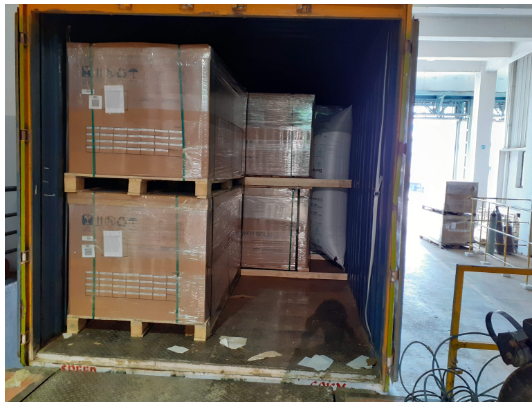
Figure 6.2: PV module pallets loaded inside the container (metal floor).
