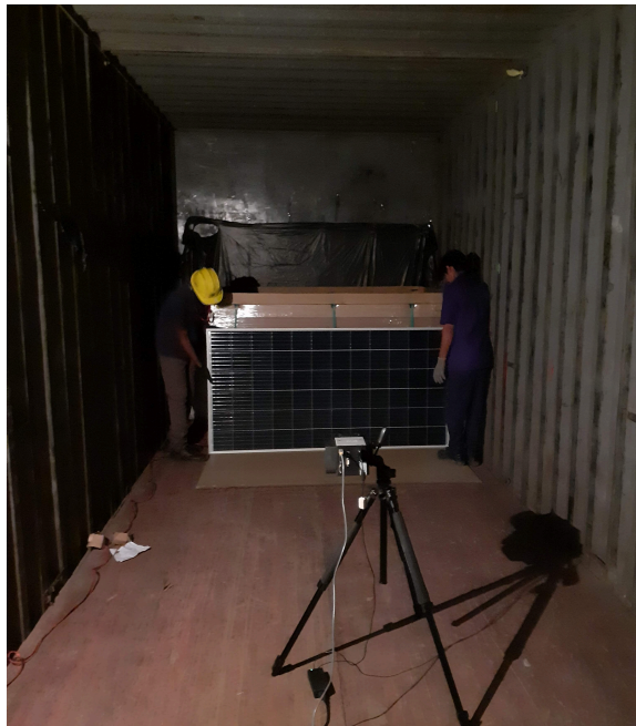
Figure 6.1: Dark room setup made for EL imaging inside the container (wooden floor).
