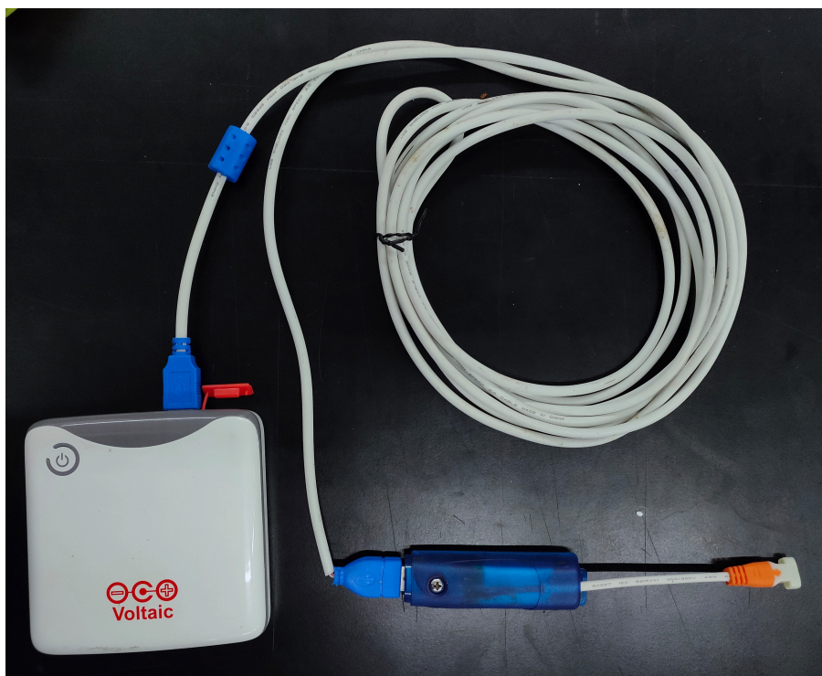
Figure 3.4: GCDC X16-4 accelerometer connected to Voltaic power bank.
