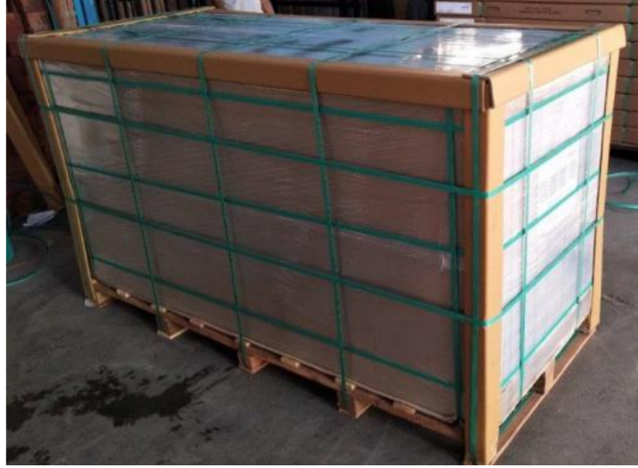
Figure 4.1: A standard pallet containing 20 PV modules.
