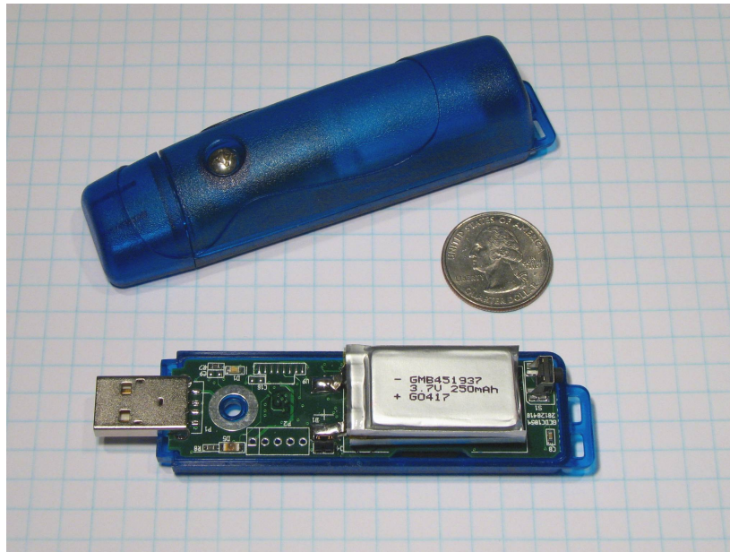
Figure 3.1: GCDC X16-4 accelerometers [6].
