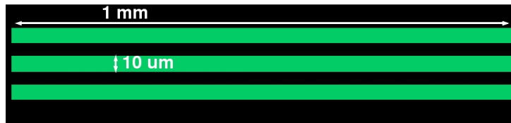
Figure 3.13: Single test patterns for contrast curve experiments. Such multiple test patterns were exposed on HSQ with varying doses in the range of 20 - 2000 \mu\text{C}/\text{cm}^2 with steps of 20 \mu\text{C}/\text{cm}^2 . Since the resist is negative tone, the green area in the pattern gets hardened on e-beam exposure and are retained after development. The black area is washed away in developer
