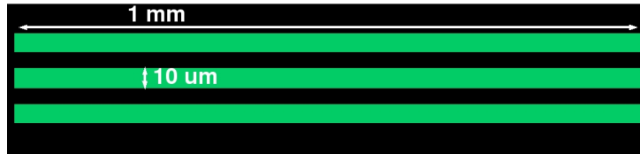
Figure 3.3: Single test patterns for contrast curve experiments. Such multiple test patterns were exposed on PMMA with varying doses in the range of 10 - 250\mu\text{C}/\text{cm}^2 with steps of 10\mu\text{C}/\text{cm}^2 . Since PMMA is a positive tone resist, cross linking happens in the green area of the pattern and gets washed away in developer. The black area is retained after development
