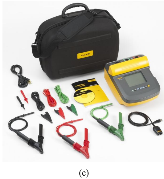
Fig. 3.7: Indoor insulation resistance characterization (a) schematic diagram of dry insulation resistance measurement setup, (b) schematic diagram of wet insulation resistance measurement setup and (c) picture of FLUKE 1550C (at NISE Gurgaon) used in field surveys.
