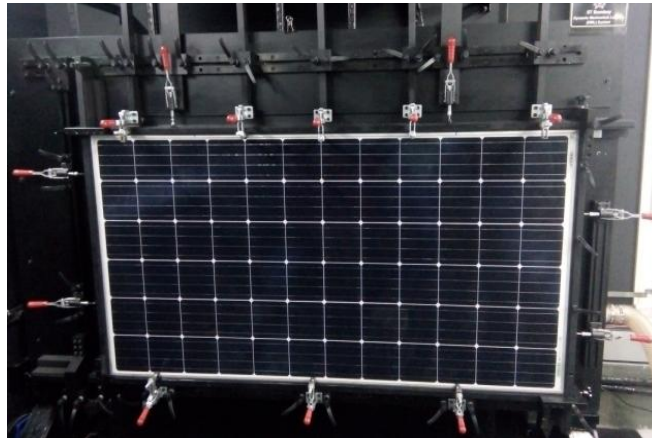
Fig. 6.3: Test module placed on the DML tool for accelerated testing.
