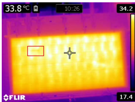
Fig. 6.20: Dark I-R (left) and EL (right) (a) for L1MoMT, (b) L1MoCB and (c) L1MuCB after 5000 cycles. Rectangle marked in red shows the similarity between the cracks in EL image and cooler region in dark IR .
