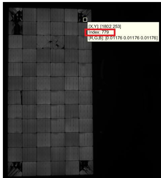
Fig. 6.8: Example for identifying threshold value in an EL image. The value marked in red represents the pixel value considered for obtaining the threshold value.
