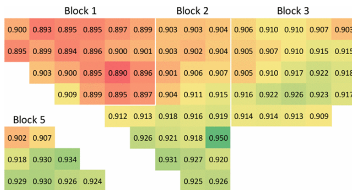
Figure 2.14: Average PR map of a PV power plant in California, USA, showing spatial variation in the PR, indicating PV soiling non-uniformity. (Reproduced from Ref. [22] © 2014 IEEE).
