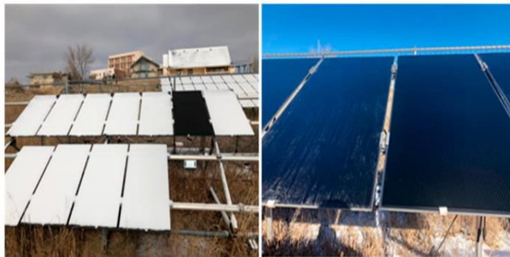
Fig. 18: (a) The black module (which is not covered with snow) was coated with a hydrophobic coating (coating A). “(b) Following the snowmelt, dust residues were deposited on the not-coated module (left), while the coated module (right) remained clean” [32].
