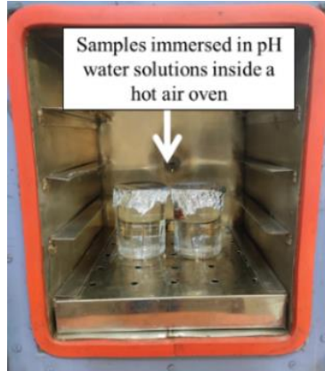
Fig. 104: Photograph of coated samples immersed in pH 6 water solution inside a hot air oven.
