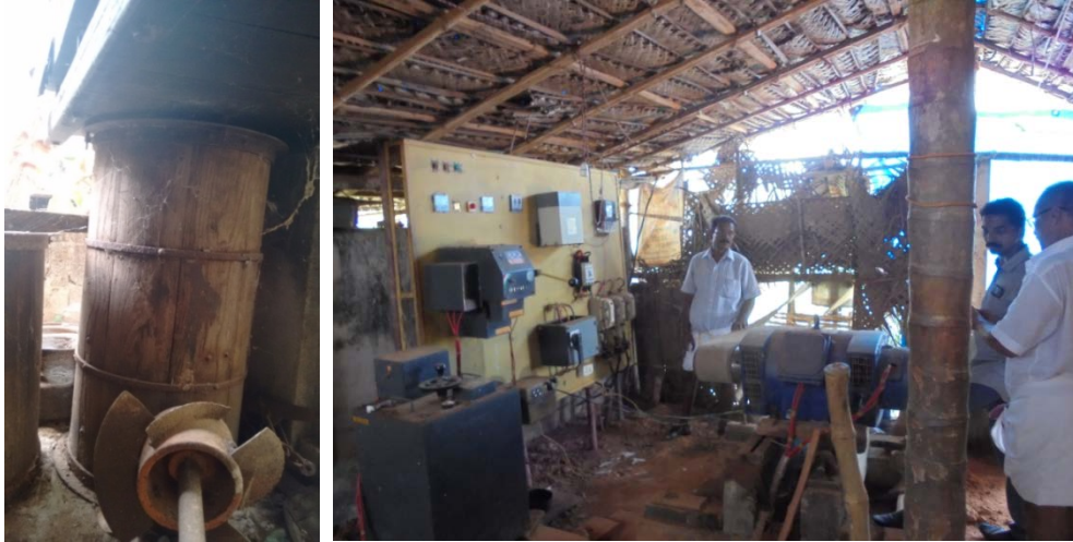
Figure 5.1: Petti and Para (wooden box and cylindrical casing) and the impellor used and the mode of driving with electric motor and belt.
