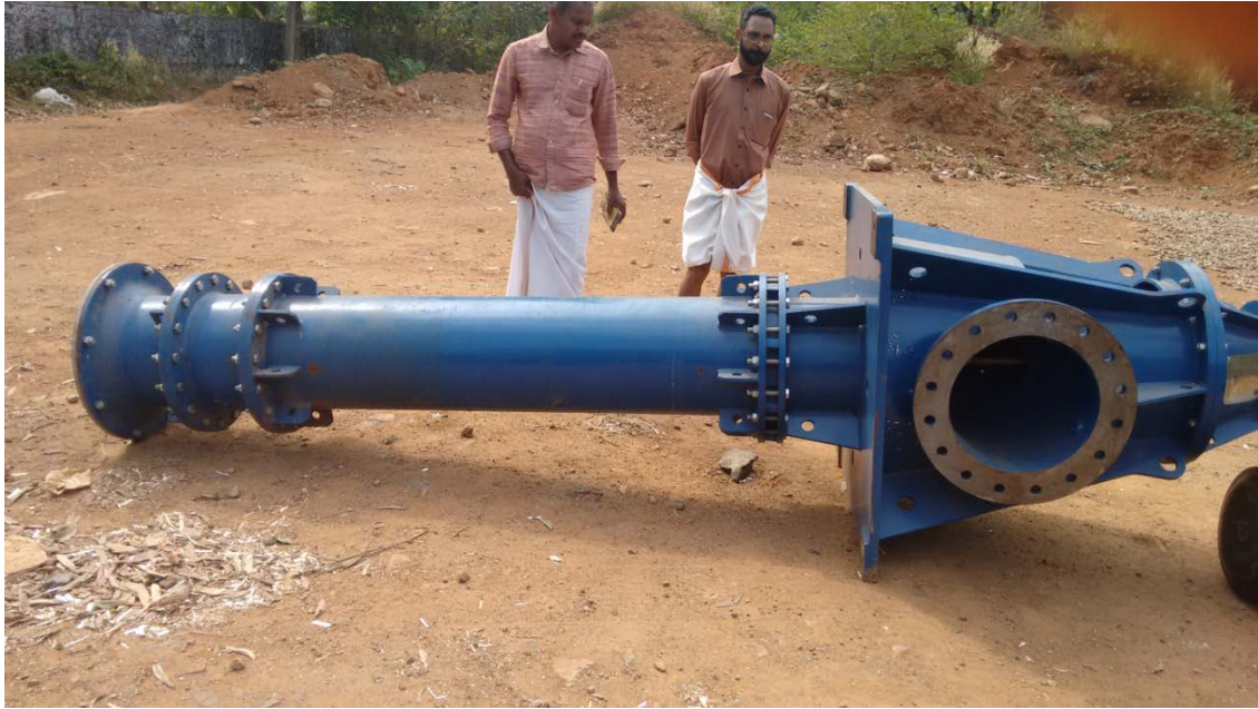
Figure 5.2: Turbine pump with 30 HP vertical mounting from Kirloskar.
