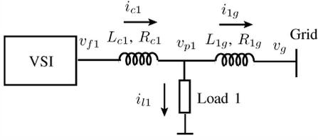
Fig. 1. Single VSI connected to the grid
