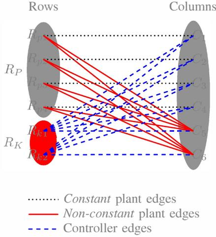
Fig. 4. Bipartite graph for single VSI connected to the grid
