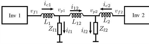
Fig. 2. Two-inverter-connected microgrid
