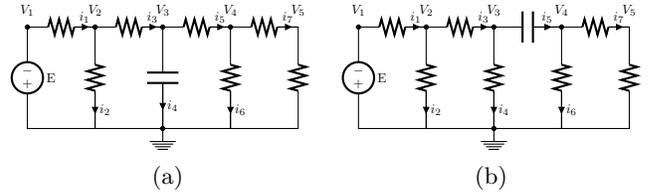
Figure 12: (a) A 5-rung resistance ladder with capacitor in parallel, (b) the capacitor in series.
