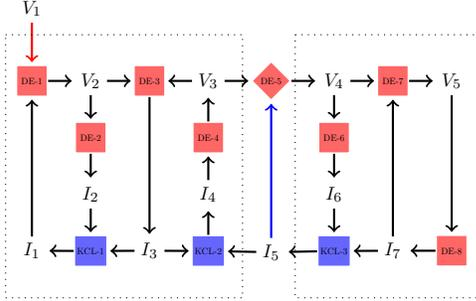
Figure 14: Directed consistent graph Example 4.1, capacitor in series removes one rung. The left block has  $C_N = F_5 = 5$  and right block has  $C_N = F_4 = 3$ , for the complete graph  $C_N = F_4 \times F_4 + F_5 \times F_3 = 19$ , where  $F_n$  is Fibonacci series.
