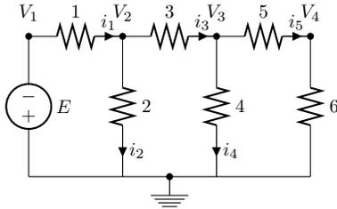
Figure 3: Resistance ladder 3-rung
