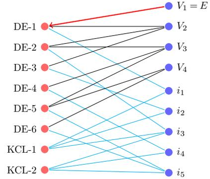
Figure 4: Separated bipartite graph (equation-variable separated)
