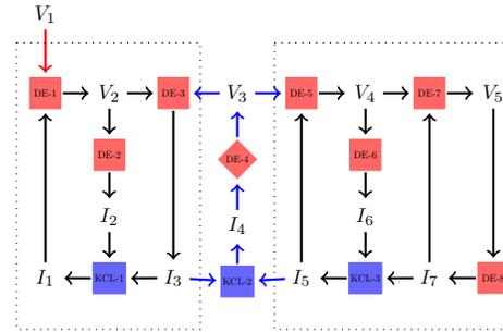
Figure 13: Directed consistent graph for Example 4.1: the capacitor divides the graph into two parts. The left block has  $C_N = F_4 = 3$  and right block has  $C_N = F_5 = 5$ , for the complete graph  $C_N = 3 \times 5 = 15$
