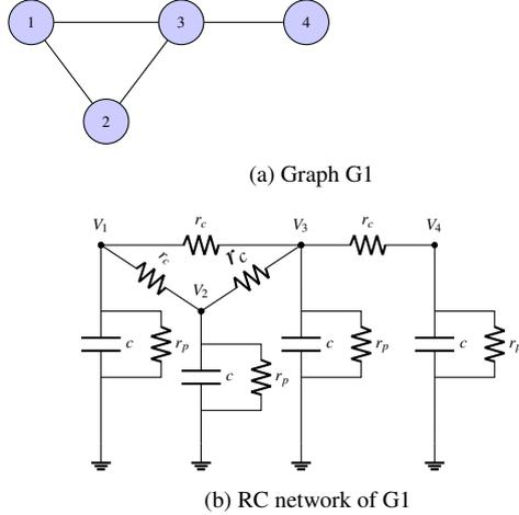
Fig. 1. Graph, multi-agent network and analogous RC circuit
