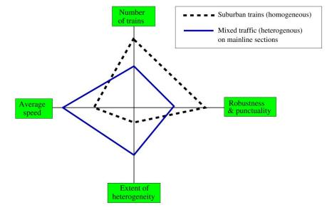
Fig 1.1: The balance of railway capacity (adapted from [11])
