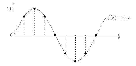
Figure 2: Sampling a sine wave
