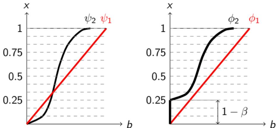
Figure: Optimal Power-allocation for  $\beta = 0.75$
