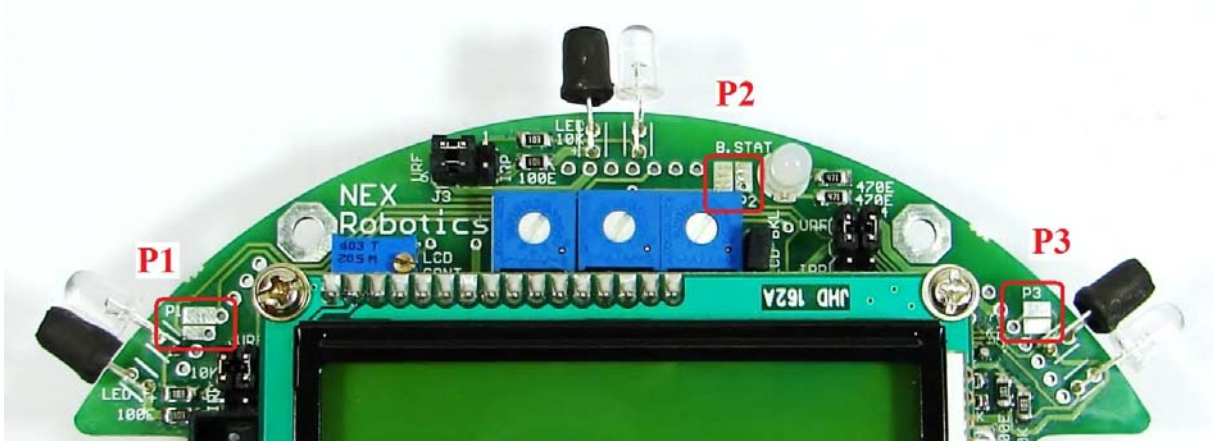
Figure 3.21: Pads for bypassing particular Ultrasonic range sensor
