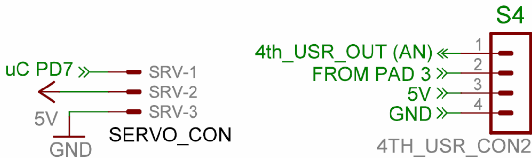
Figure 3.40: Servo motor and sensor connections
