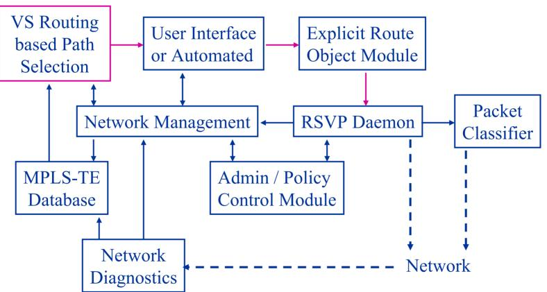
Using Virtual Space (VS) routing for MPLS-TE optimization
