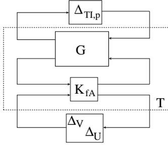
Fig. 6. Plant and controller interconnection for coprime factor reduction
