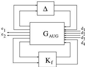
Fig. 7. The Augmented Plant and Controller
