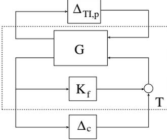
Fig. 4. Plant and controller interconnection for additive reduction
