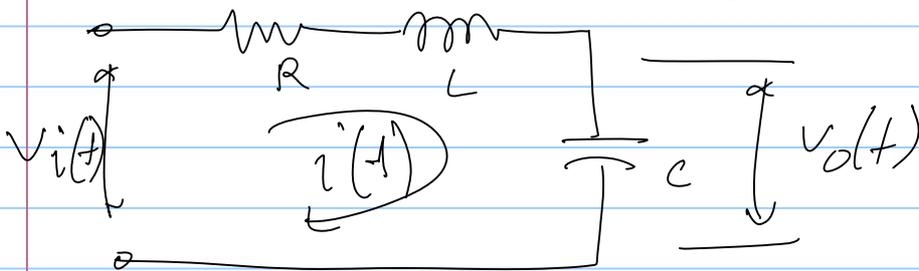
$$LC \frac{d^2 v_o}{dt^2} + RC \frac{dv_o}{dt} + v_o(t) = v_i(t)$$
