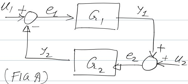
$$e_1 = u_1 - y_2, \quad e_2 = u_2 + y_1, \quad y_1 = G_1 e_1, \quad y_2 = G_2 e_2$$
