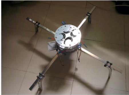
Figure 2.1: Aeroquad Cyclone frame
