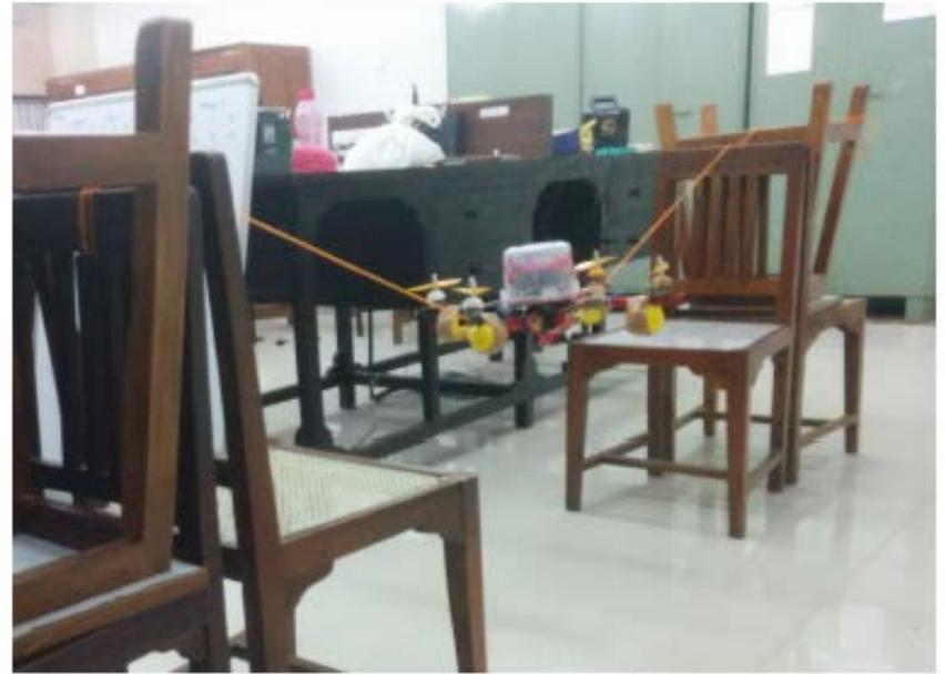
Figure 3.7: Experimental setup for Attitude mode gain tuning
