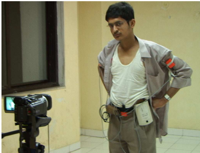
Fig. 1. Illustration of the experimental setup. Motion trackers (small orange objects) are strapped on the upper arms and the waist. The bigger object hanging at the waist where the left hand touches is the bluetooth interface for motion sensors. The single lead ECG recorder is attached to the front right side of the waist. The entire experiment is recorded on video to capture stray events not recorded by the motion sensor.
