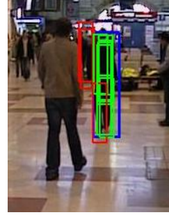
Figure 2. Figure showing outlier elimination. The fragments in red are the outliers. The fragments in green are used for localising the target. The box in blue decides the outliers.
