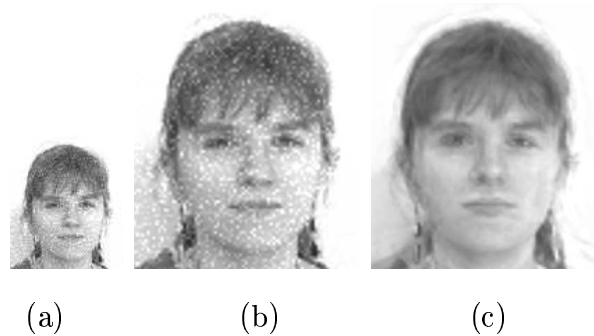
Figure 6.8: Restoration of an input image not present in the database. (a) Noisy observation, (b) bicubic interpolated image, and (c) result of PCA-based restoration for q = 2 .
