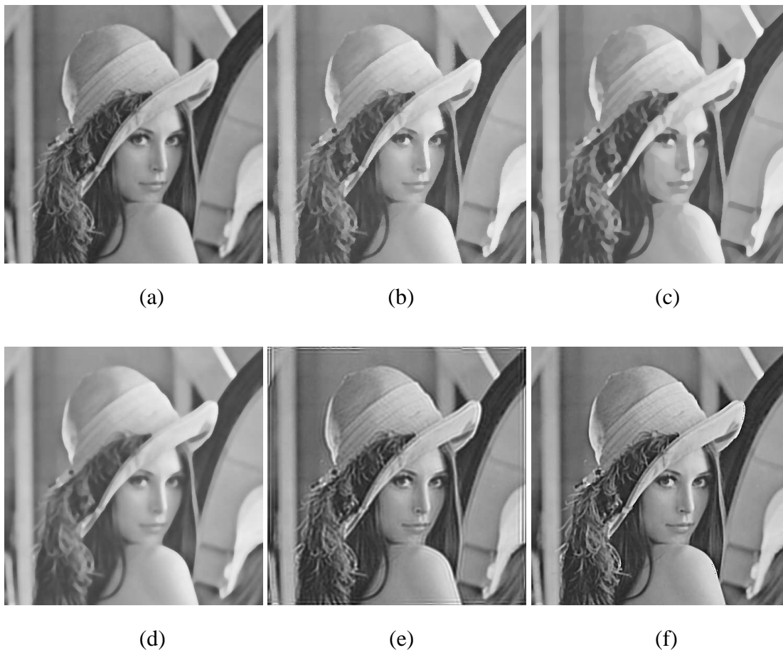
Figure 6.7: Result of inverse diffusion of the Lena image which has been blurred as shown in (a) using (b) Osher-Rudin shock filter, (c) Alvarez-Mazorra shock filter, (d) Gilboa et al. complex shock filter, (e) blind deconvolution, and (f) the proposed method.
