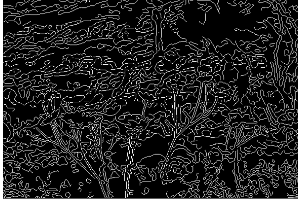
Figure 8.3: The binary valued edge map obtained using Canny edge detector that is included in the data likelihood for the scene shown in fig.8.1(a).
