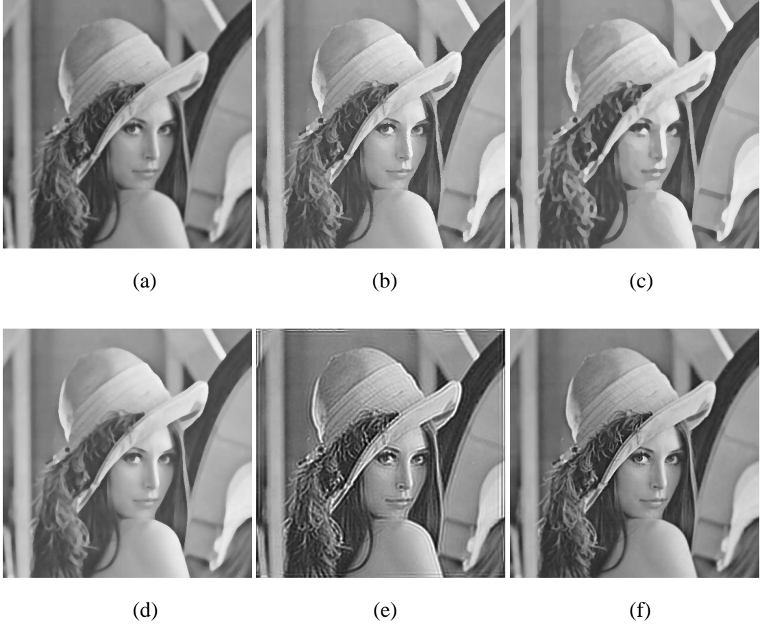
Figure 6.8: Result of space varying blind deconvolution with (a) input image using (b) Osher-Rudin shock filter, (c) Alvarez-Mazorra shock filter (d) Gilboa et. al complex shock filter, (e) blind deconvolution and (f) using the proposed method.
