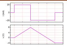
Plot v, p, and W versus time 20 for the given source current. Assume v(0)=0 V, C=5 mF. i (mA) 0 -20 8 4 Ś
