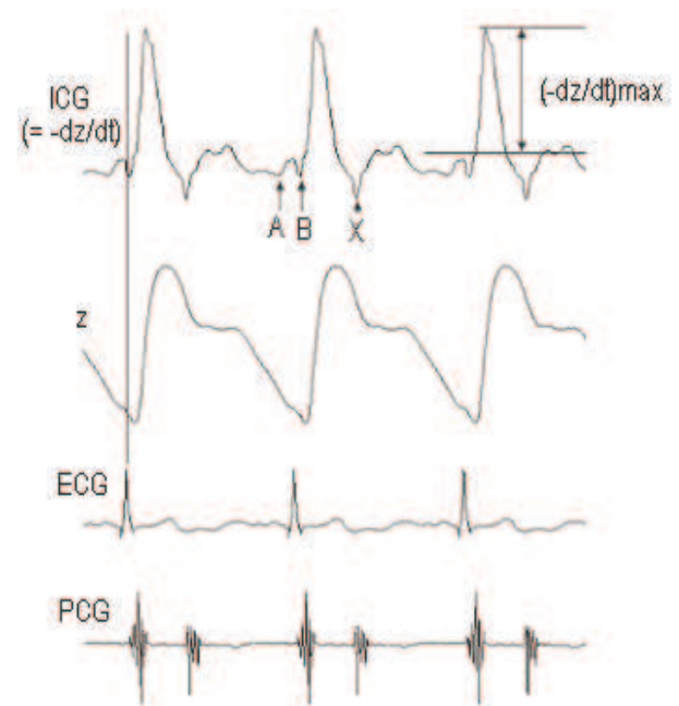
Fig. 1 Typical impedance cardiogram (adapted from [9]). z(t) = Z_o - Z(t) where Z(t) is thoracic impedance and Z_o is the basal impedance.
