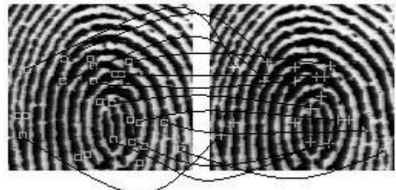
Figure 11. Matching between two impressions of the same finger. Both the images have been locally captured. 16 of the 24 minutiae in the left image match 16 of the 18 minutiae in the right image.
