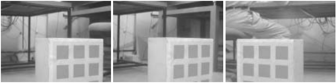
Figure 5.5: The sequence of images used for special case 2 of pose estimation (Section 5.3.3): constrained rotation about the Y -axis only
