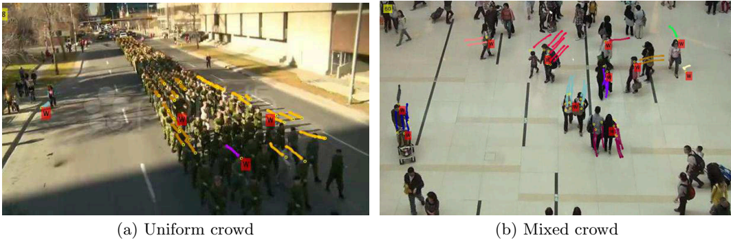
Figure 1: Output of the our proposed group detection algorithm: (a) and (b) give examples of structured and unstructured crowd. Tracklets for some of the agents over past few frames are also shown. Each color represents a group (Best viewed in color). The videos are from CUHK [14] datasets
