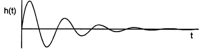
Fig. 7. Simulated impulse response  $h(t)$  of the transducer.
