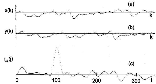
Fig. 9. Results of cross correlator simulation. (a) turbulence signal  $x(k)$  obtained at upstream sensor; (b) Turbulence signal  $y(k)$  obtained at downstream sensor; (c) cross correlator output  $r_{xy}(j)$ .
