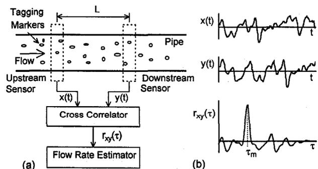
Fig. 1. Schematic of flow measurement by cross correlation technique. (a) Block diagram of cross correlation flowmeter; (b) signals  $x(t)$  and  $y(t)$  obtained at the two sensing locations, and their cross correlation function  $r_{xy}(\tau)$ .
