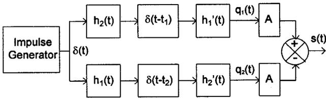
Fig. 6. Model of ultrasonic pulse transmission and reception.
