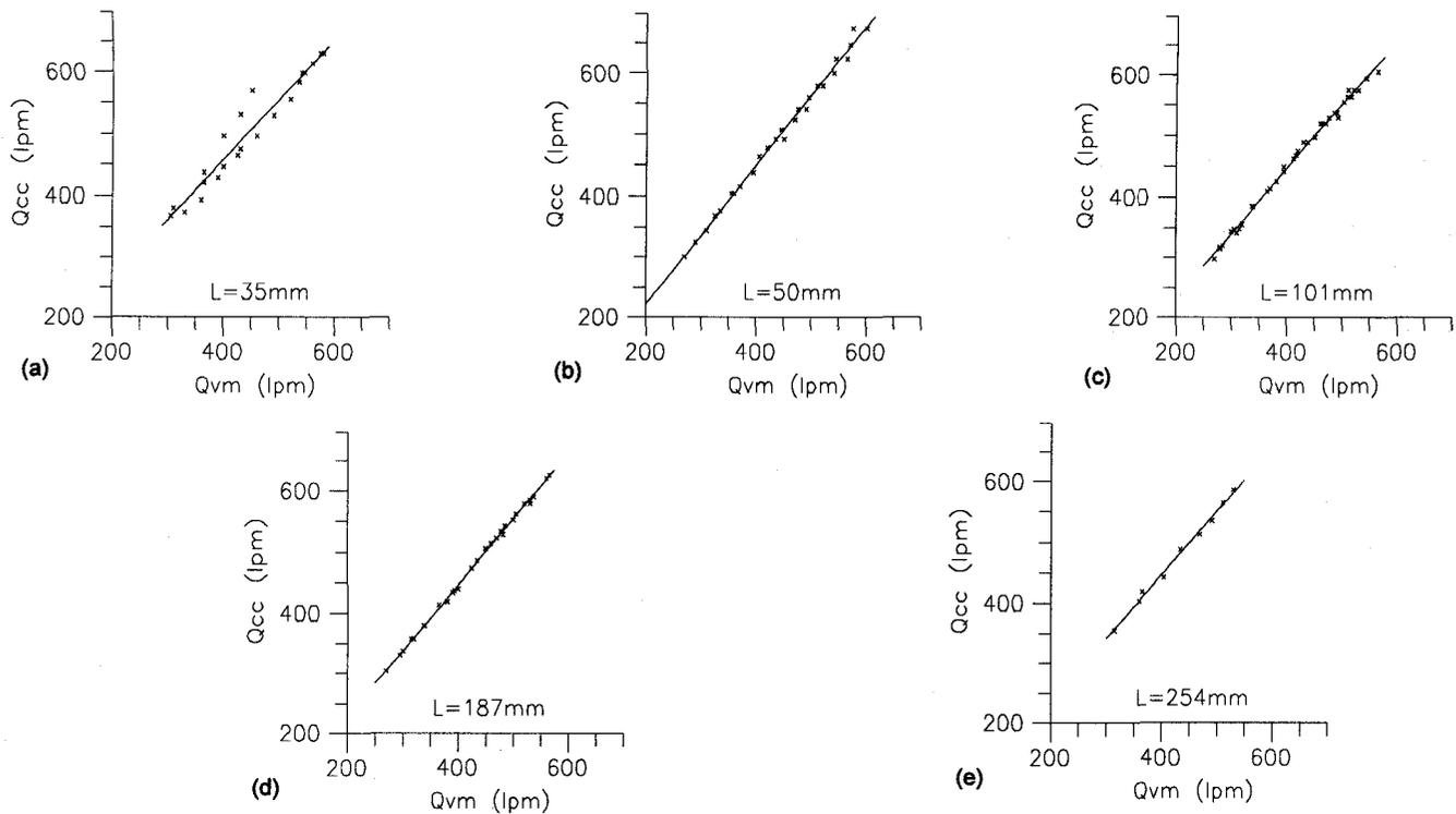
Fig. 11. Graphs of flow calculated by cross correlation technique ( $Q_{cc}$  in lpm) versus flow measured by venturimeter ( $Q_{vm}$  in lpm) for various sensor spacings ( $L$ ): (a) 35 mm; (b) 50 mm; (c) 101 mm; (d) 187 mm; (e) 254 mm.
