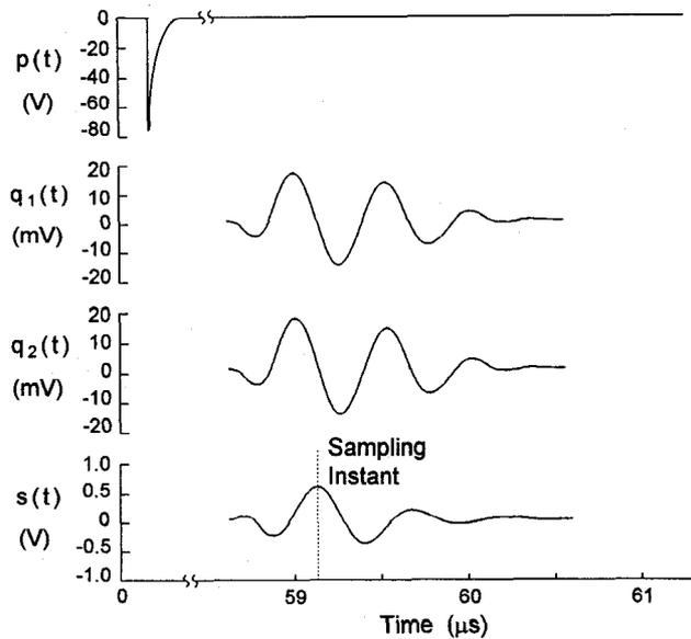
Fig. 3. Waveforms showing excitation pulse  $p(t)$ , received pulses  $q_1(t)$  and  $q_2(t)$ , and differential amplifier output  $s(t)$ .
