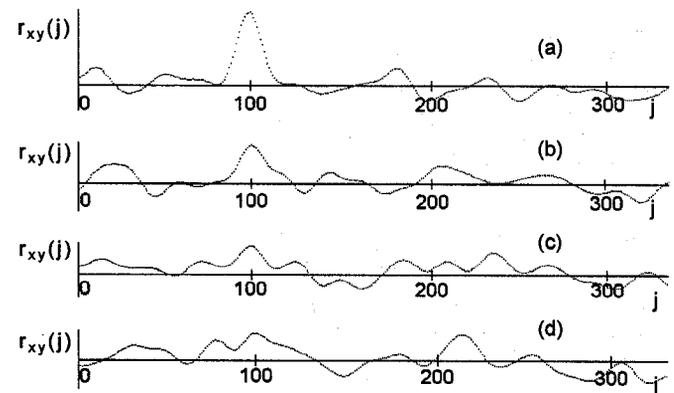
Fig. 10. Cross correlator output with random noise added in the turbulence signal obtained at the downstream sensor. Amount of noise added: (a) 100%; (b) 200%; (c) 300%; (d) 400%.
