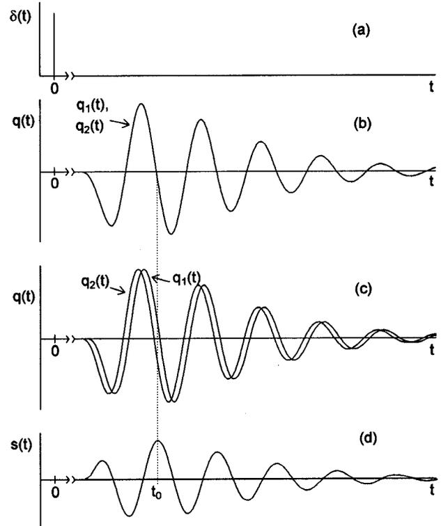
Fig. 8. Results of simulation of the model given in Fig. 6. (a) shows the excitation impulse  $\delta(t)$ . The Receiver outputs  $q_1(t)$  and  $q_2(t)$  as shown in (b) arrive at the same instant at zero flow. Receiver outputs and differential amplifier output  $s(t)$  in the presence of a turbulent velocity component are shown in (c) and (d) respectively.  $t_0$  indicates the sampling instant.
