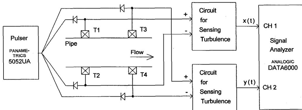
Fig. 5. Block diagram of the experimental set-up for flow measurement by cross correlation technique.
