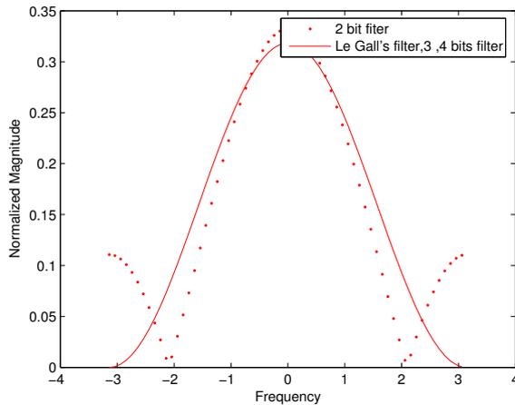
Figure 4: frequency responses of G0 filters at various wordlengths
