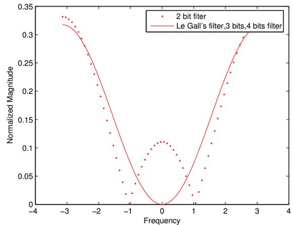
Figure 3: frequency responses of H1 filters at various wordlengths
