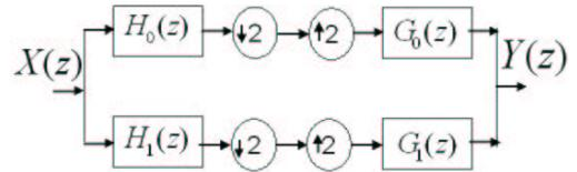
Figure 1: Block diagram of two band filter bank
