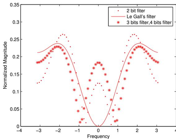
Figure 5: frequency responses of G1 filters at various wordlengths
