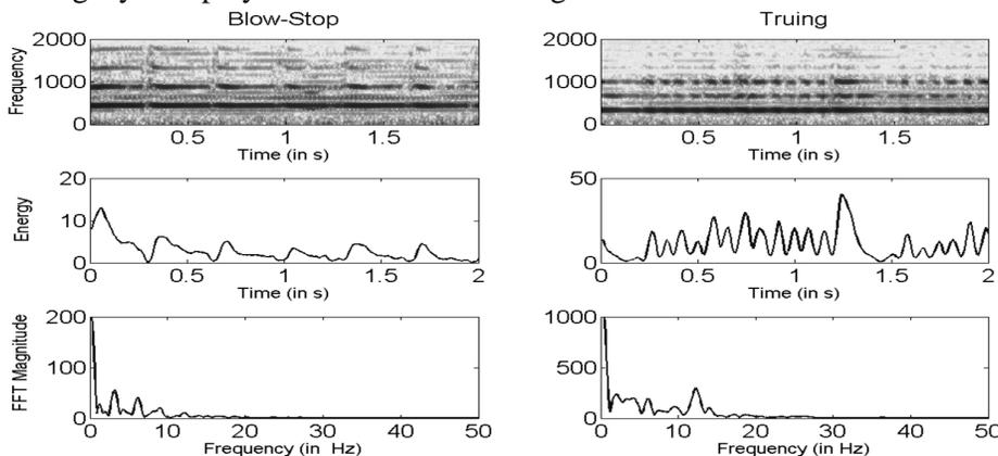
Figure 2: Depiction of spectrogram variations along with the energy contour and the 1024-pt FFT on chunks of size 2s for blow-stop (on left) and Truing(right).
