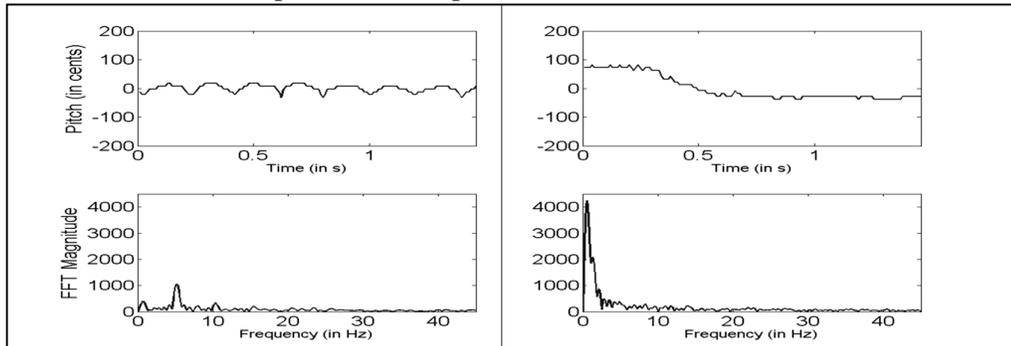
Figure 1: Comparison of 1024-pt FFT of 1.5s chunk of data for vibrato characteristics
