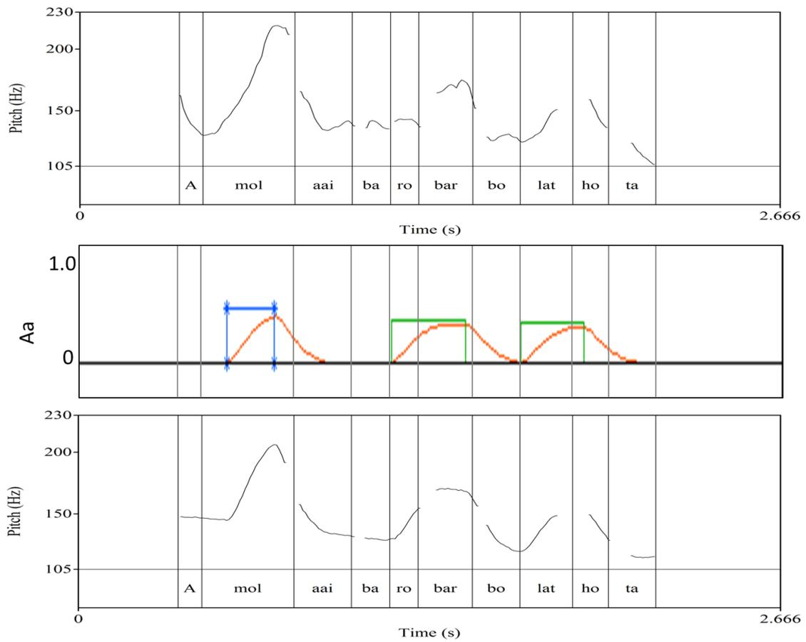
**Figure 10: Different stages in the combined manipulation of duration and F0 contour of the utterance (from top to bottom: the original syllable segmentation, the desired duration scaling contour, the modified syllable segmentation, the extracted F0 contour of the duration modified utterance, the corresponding Fujisaki model accent commands, the manipulated accent commands, and the resulting final manipulated F0 contour)**
