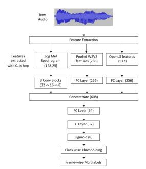
Fig. 3: 3-branch architecture of the frame-based classifier
