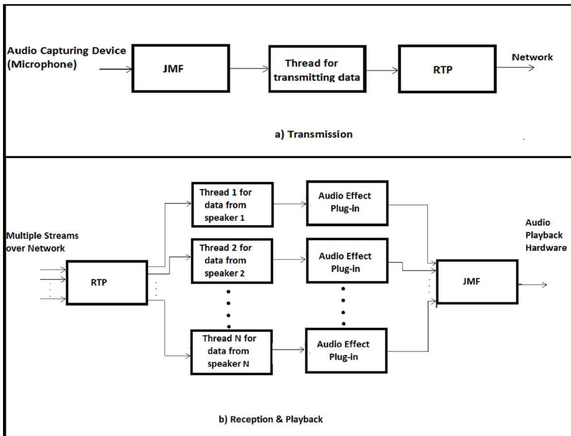
Figure 6.a) Block diagram for for the transmission part
