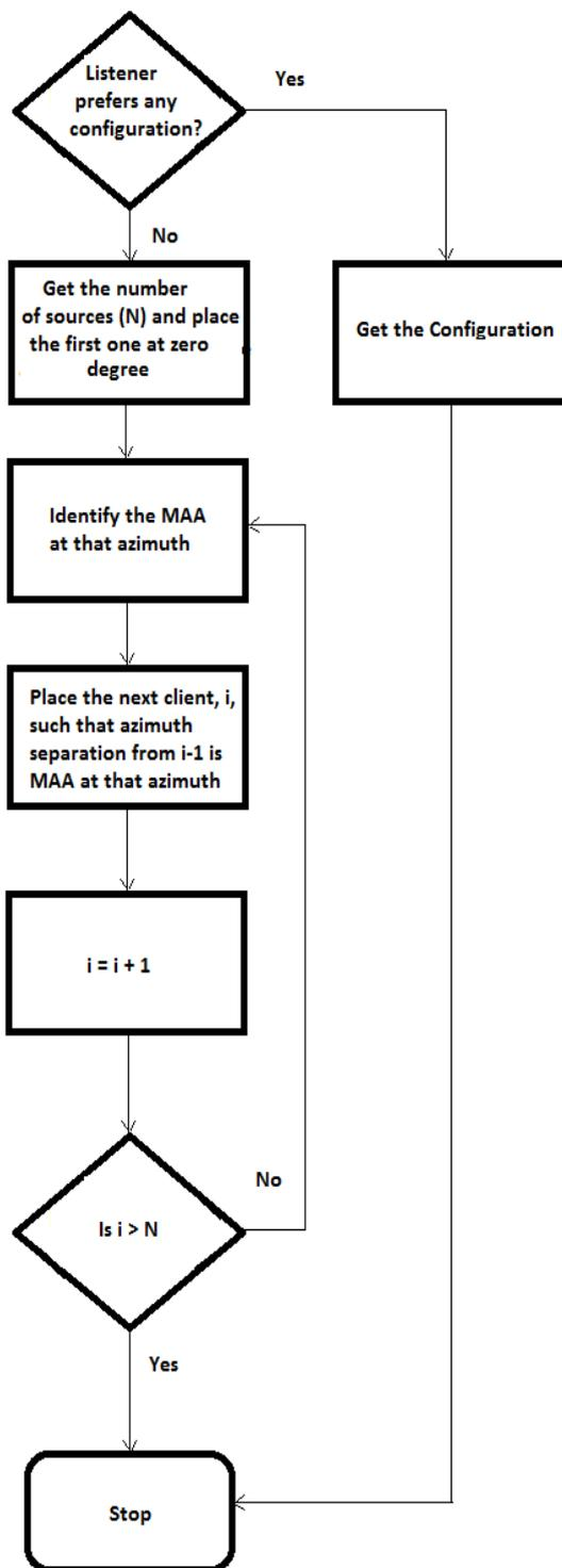
Figure 1. Flow chart representation of the speaker placement algorithm
