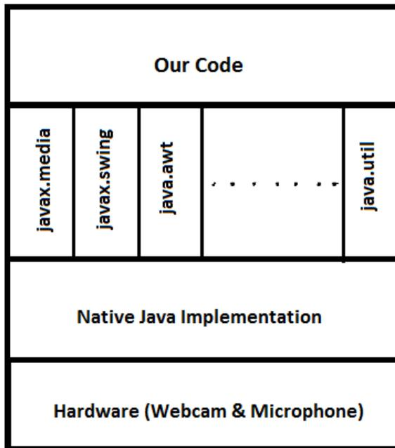
Figure 5. The layered architecture of each client
