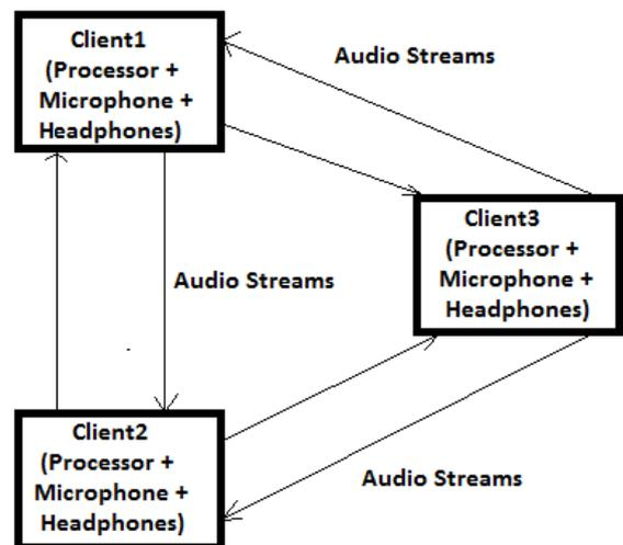
Figure 4. Overall architecture for the 3 participant case. Mono audio streams are transmitted between clients.
