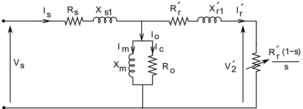
Figure 1: Per phase equivalent circuit of Induction Motor
