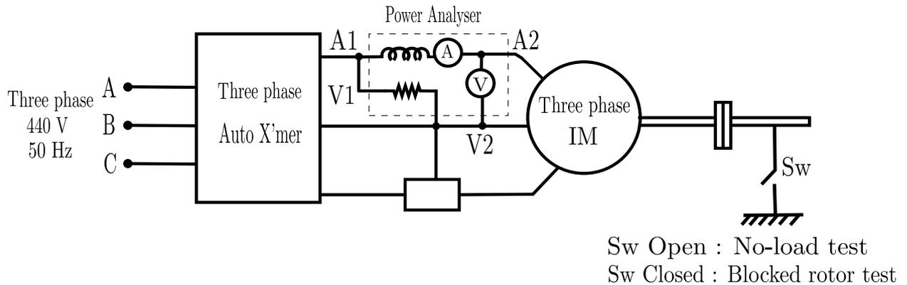
Figure 2: Circuit Diagram for no-load and blocked-rotor test on 3 Phase Induction Motor
