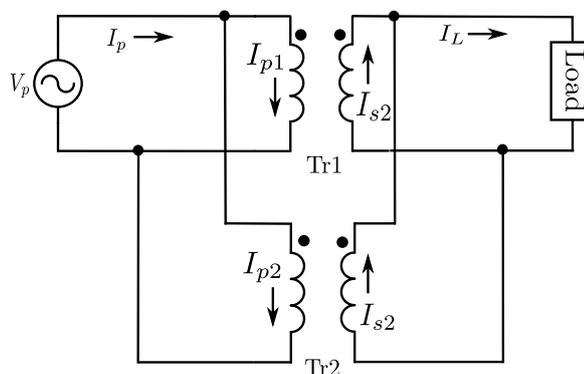
Figure 1: Conceptual Diagram of Two single-phase Transformers in Parallel
