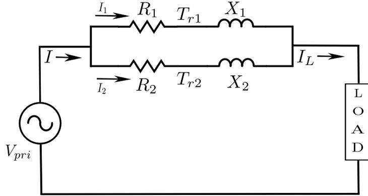
Figure 2: Equivalent Circuit of Two Single-phase Transformers in Parallel
