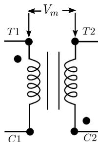
Figure 1: Single phase transformer
