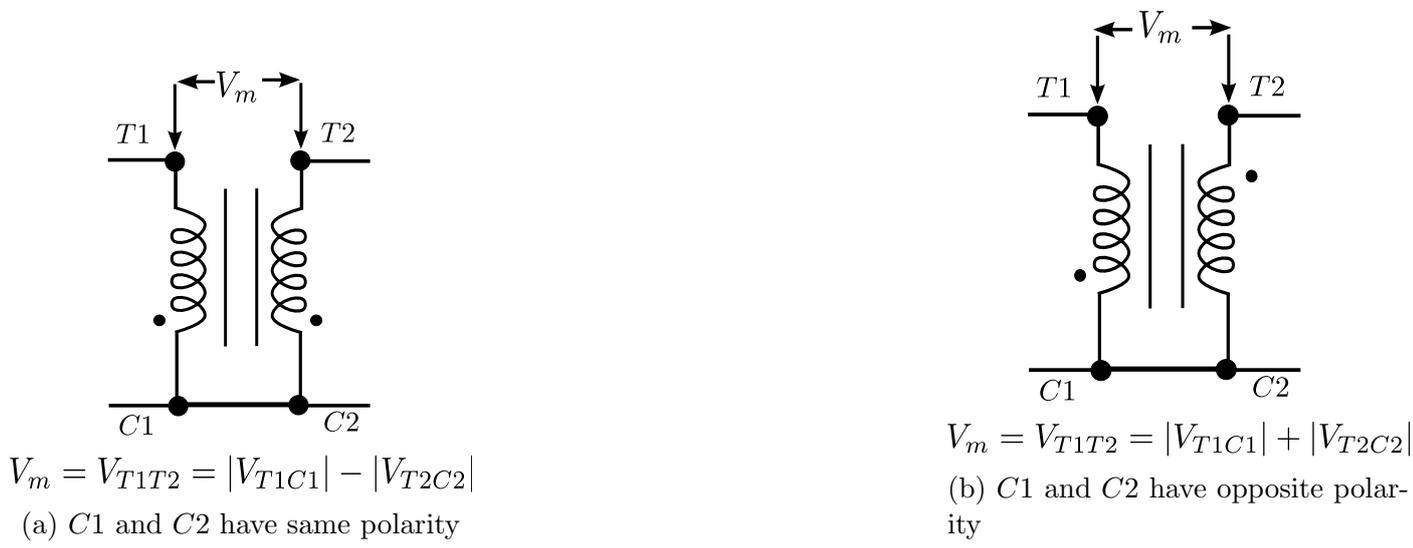
Figure 3: Expected outcome of polarity test
