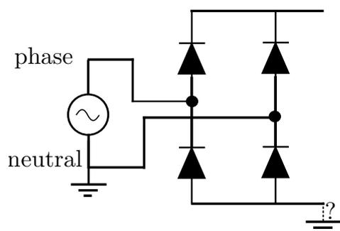
Figure 4: Proposed connections for single phase DC supply
