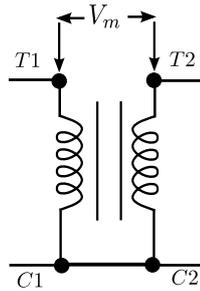
Figure 2: Connections for polarity test
