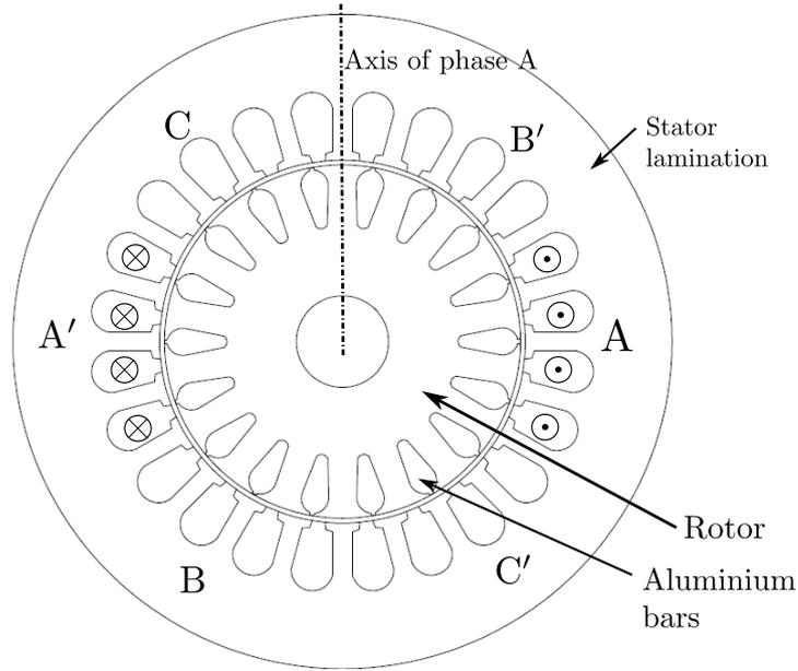
Figure 2: Distributed coil arrangement for 2 pole 3 phase induction machine
