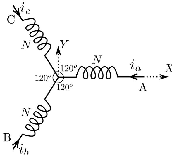
Figure 1: Coil arrangement to produce rotating magnetic field
