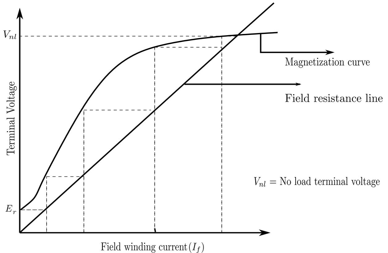
Figure 1: Voltage buildup in self-excited generator
