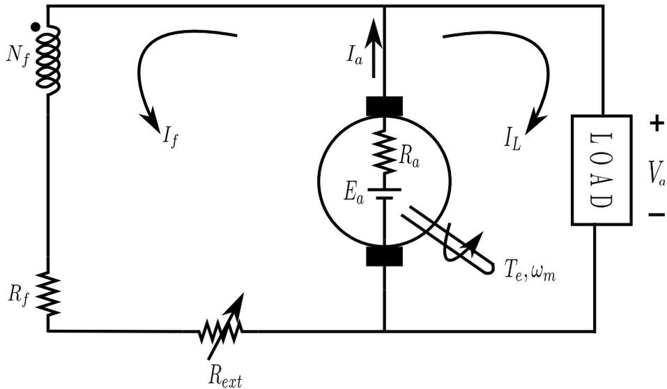
Figure 2: An equivalent circuit of self-excited DC generator
