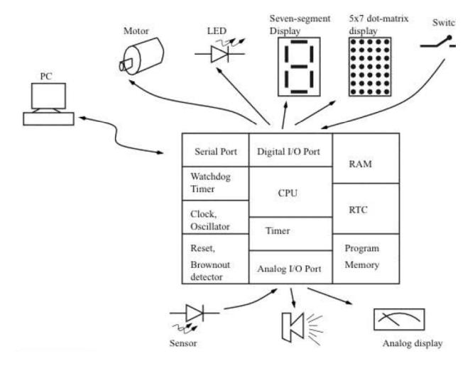
A microcontroller interfaces to external devices with a minimum of external components
