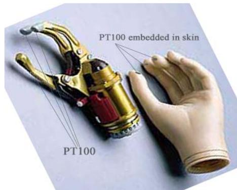
Fig 3: Artificial hand showing PT100 position
