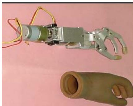
Fig 1: A Picture of the Dual Motor Prosthetic Hand and Glove, developed at *IIT Bombay* and *CMC Vellore* [1]
