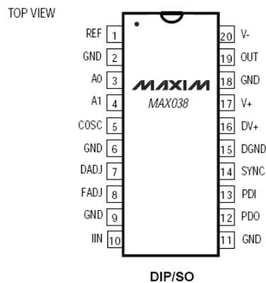
Fig. 15 Pin Diagram of MAX038
