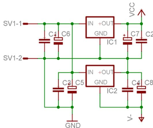
Fig. 14 Regulated Power Supply
