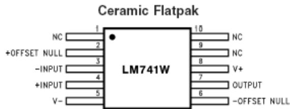
Fig. 17 Pin Diagram for LM741 OPAMP
