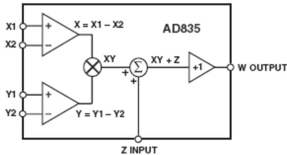
Fig. 8 Functional Block Diagram of AD835
