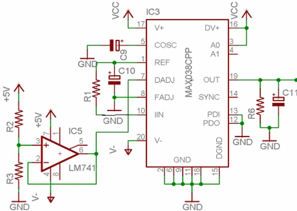
Fig.2 Circuit Diagram for 4V p-p sweep generator
