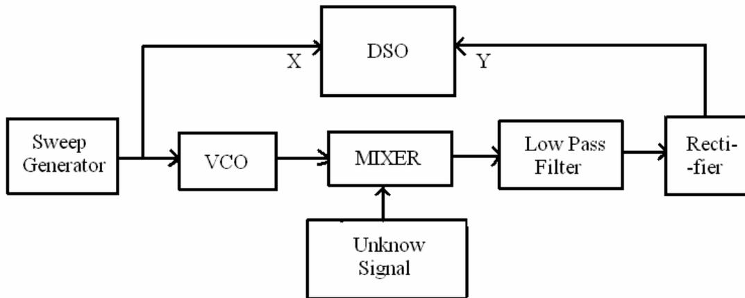
Fig. 1 Functional Block Diagram of Spectrum Analyzer
