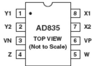
Fig. 16 Pin Diagram of AD835
