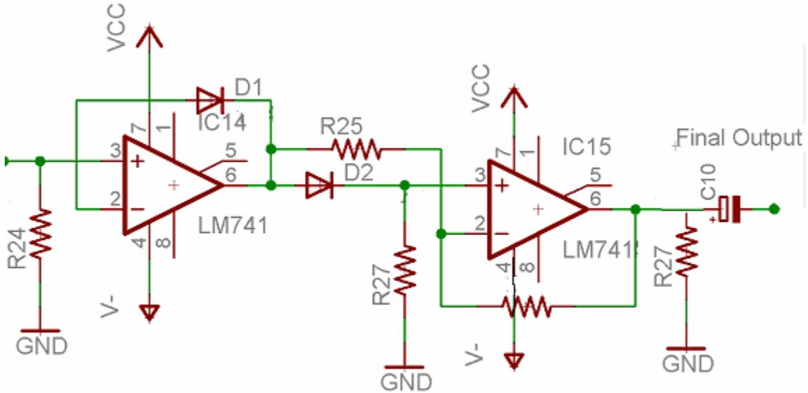
Fig. 13 Output Rectifier and Peak Detector
