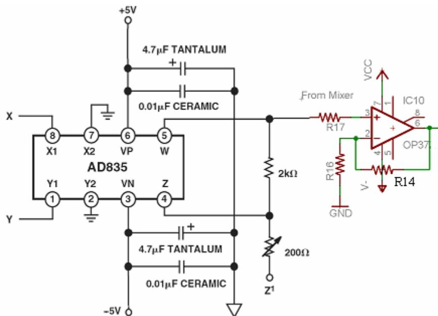
Fig. 9 Multiplier connections
