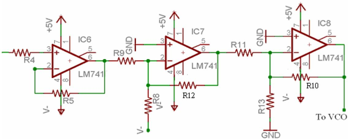
Fig. 4 Voltage adder for sweep
