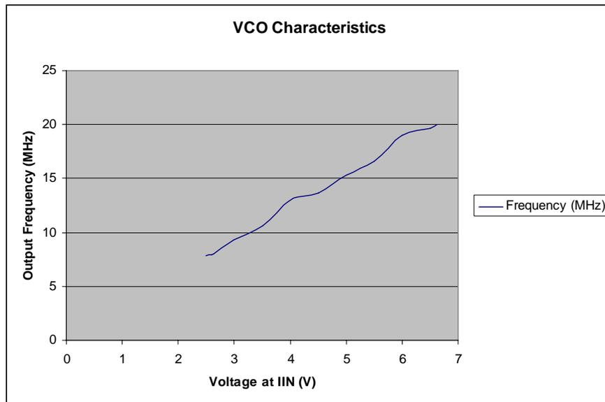
Fig. 7 VCO Output Characteristics
